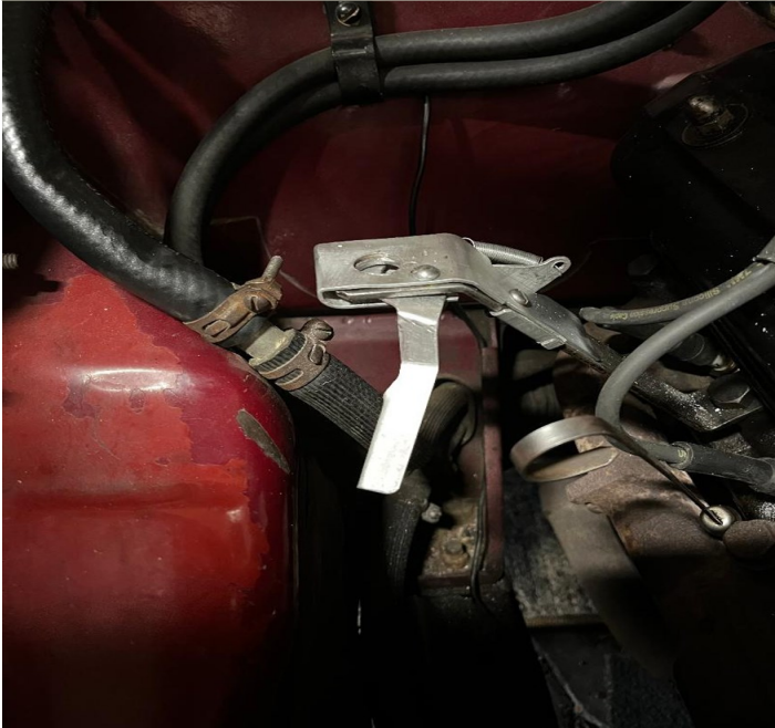
With a locked nut on bottom of the screw that holds the bowl, You push the latch, the hole opens. Spring holds it shut. Saves time and labor the once every two years he needs the air cleaner removed.
