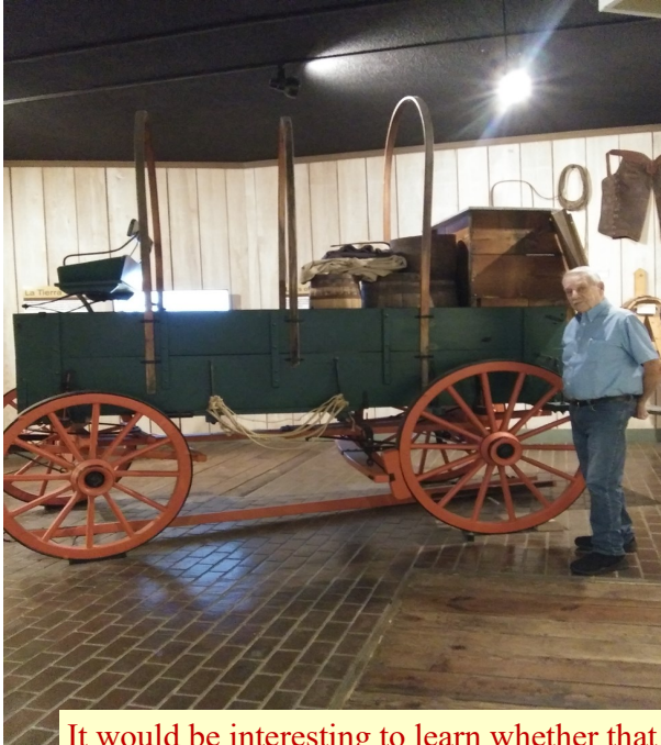
The smaller front wheels allowed more play as their axle turned with the mules.
